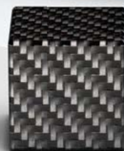
CRP / GRP / aramid Polymers with fibre reinforcement, note Tg and fibre orientation .
